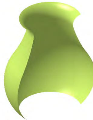
Figure 9-12 Surface revolved through an angle of 180-degree
